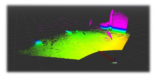
The 2 cameras can generate a very dense point cloud of the rovers' surroundings even in no-light condition.
